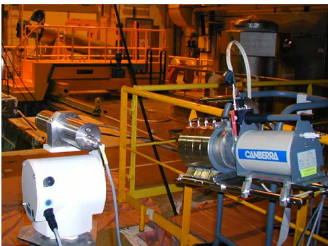
Figure 6. At the left the CAROGAM finds sources, at the right the ISOCS qualitatively and quantitatively measures radioactive isotopes
