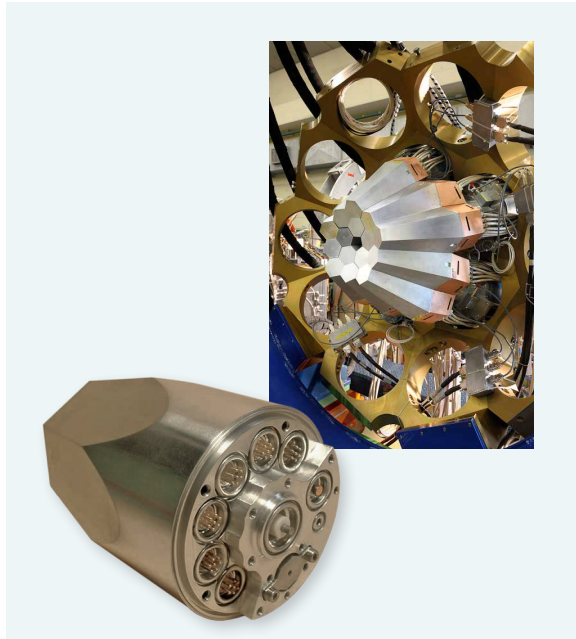
AGATA detector and the AGATA demonstrator at Legnaro consisting of the first five triplet detectors.
