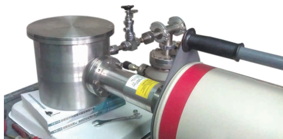
ESLB-X detector connected on a vacuum chamber. The ESLB-X is consisting of a portable slimline cryostat Big MAC type with a 7 liter Dewar.
