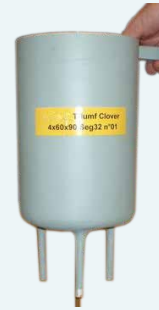
LN 2 filling funnel for manual filling in vertical position
