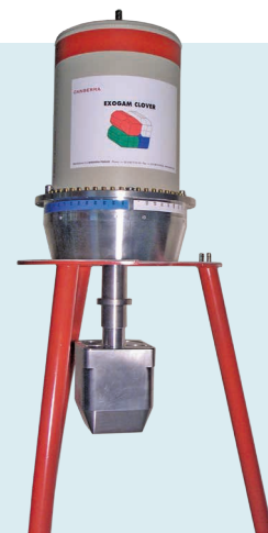
EXOGAM type Clover detector 4x60x90-seg16 with back catcher cryostat
