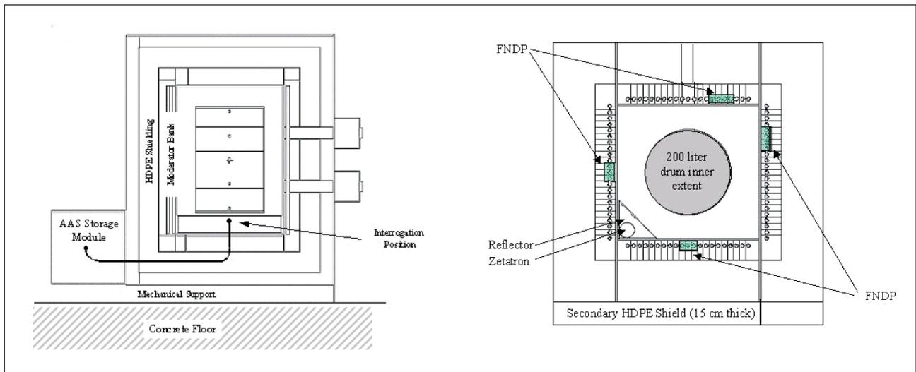
**Figure 1.** Sketch of the layout of the IWAS assay cavity. The figure at left shows the AAS source interrogation position in the center of the rotator assembly. The figure at right shows the location of the four fast Cd covered neutron detection packages (FNDP).
